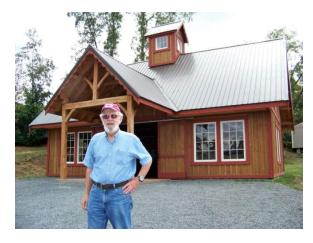
Victorian frills on the outside. The beams have hand-cut, mortise-and-tenon joints, held together with wooden pegs, just like in days gone by. The antique 12-pane windows allow lots of natural light as well as outside viewing of the carriages when the doors are closed.
